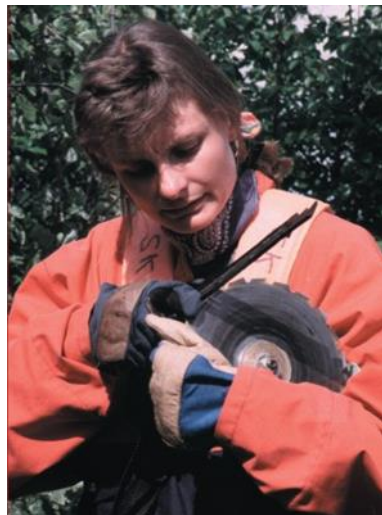
A good working position when filing, setting and changing of blades is important.
